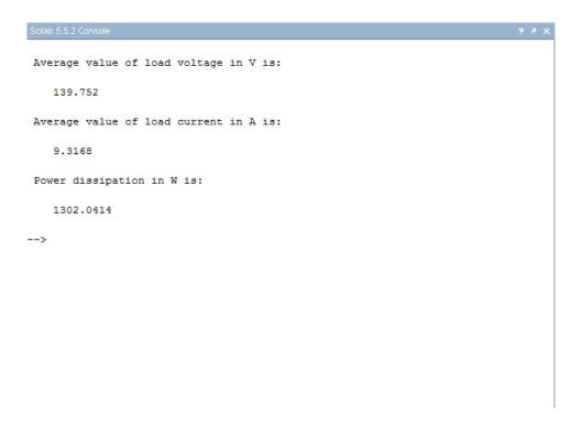
Figure 3.10: Determine the average value of load voltage and current and power dissipation  ${\bf r}$
