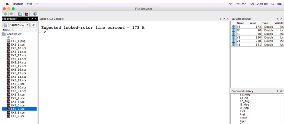
Figure 5.7: Determine expected locked rotor line current
