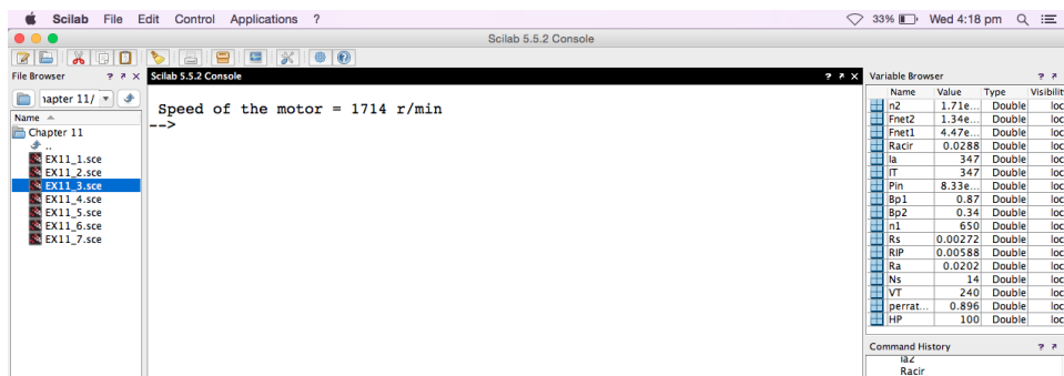
Figure 11.3: Computation of Speed if the load is reduced to a value that causes the armature current to be 30 percent of the rated current
