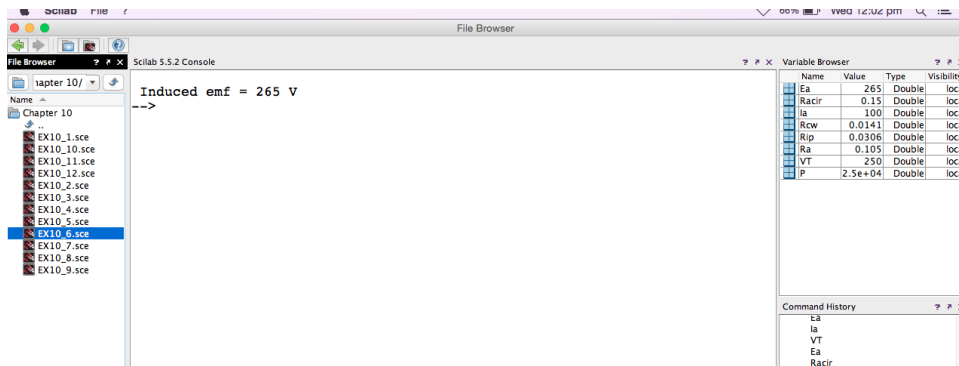
Figure 10.6: Computation of Induced emf
