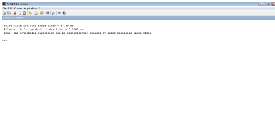
Figure 2.3: To compare \Delta T for step index fiber with parabolic index fiber
