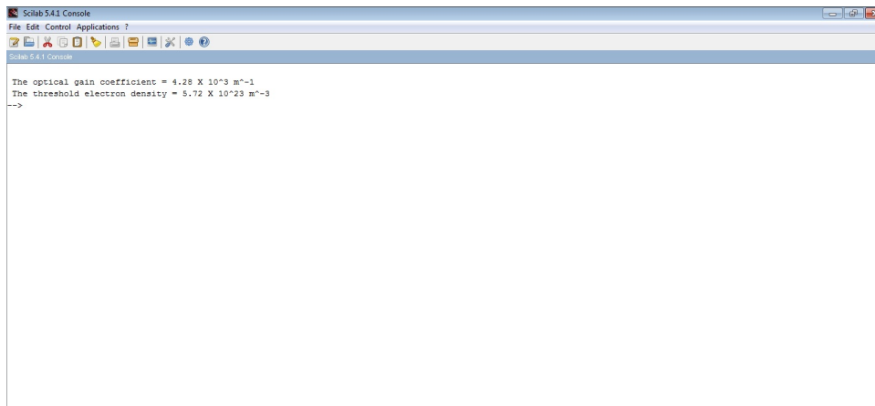
Figure 3.11: To calculate the optical gain coefficient required to balance the cavity loss and the threshold electron density N_e
