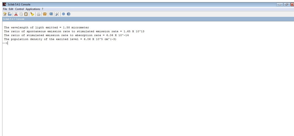
Figure 3.2: To calculate the wavelength of light emitted the ratio of spontaneous emission rate to stimulated emission rate the ratio of stimulated emission rate to absorption rate and the population density of the excited level
