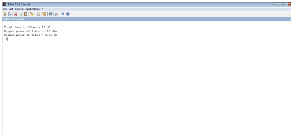
Figure 2.6: To find the total loss and output power in mW and dBm in fiber
