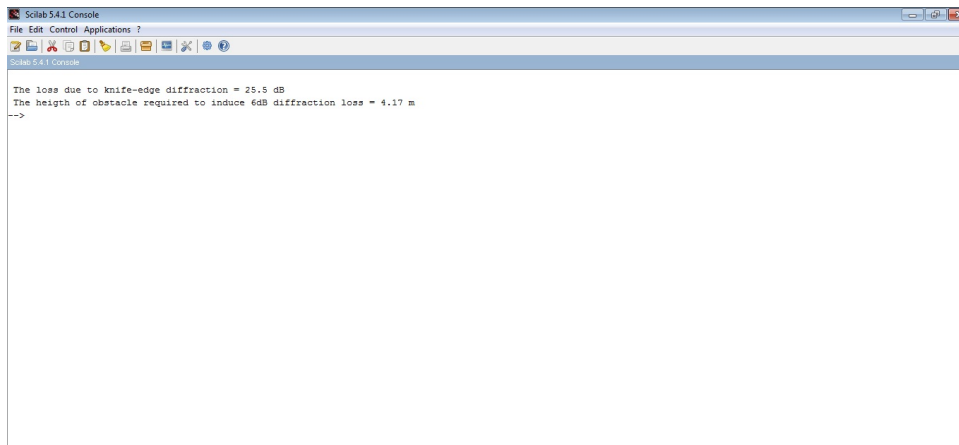
Figure 4.7: To determine the loss due to knife edge diffraction and the height of obstacle required to induce 6dB diffraction loss
