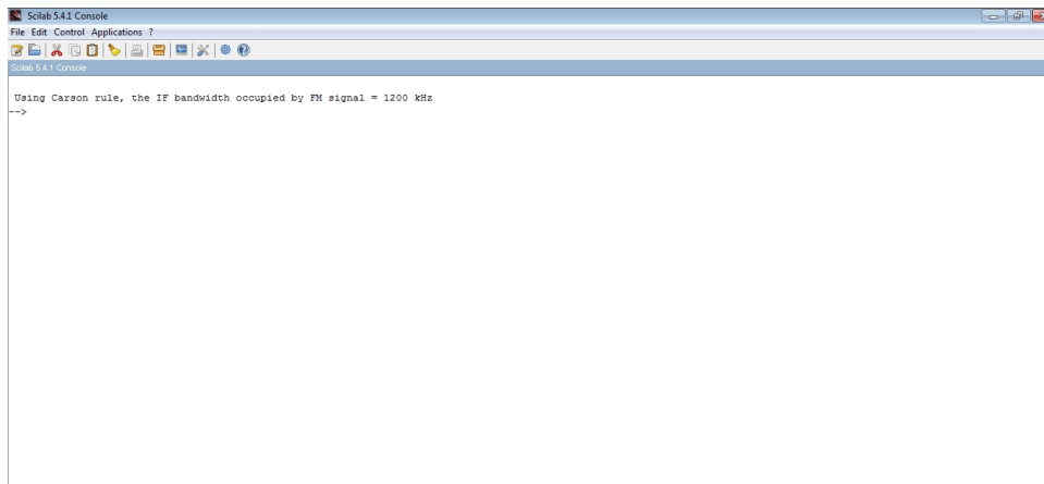
Figure 6.3: To determine the IF bandwidth necessary to pass the given signal
