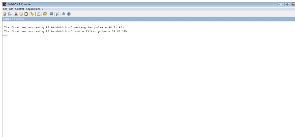
Figure 6.9: To find the first zero crossing RF bandwidth of rectangular pulse and compare to raised cosine filter pulse
