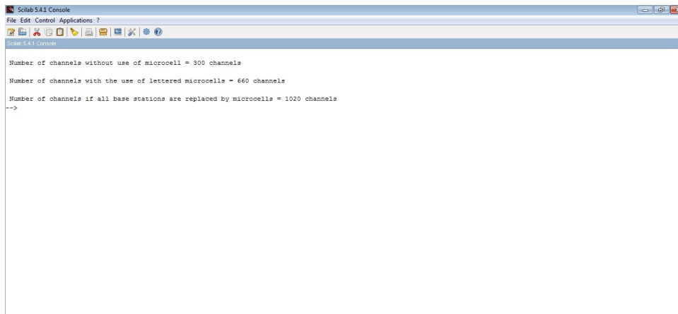
Figure 3.7: To find number of channels in 3 km by 3 km square centered around A in given Figure for without use of microcell with the use of lettered microcells and all base stations are replaced by microcells
