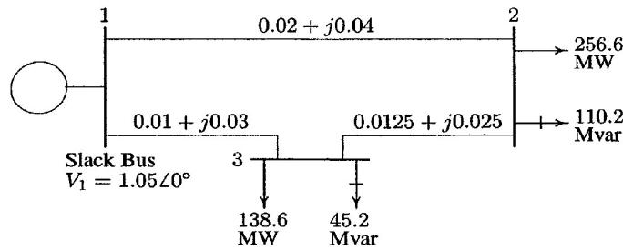
Determine the bus voltages and angle of all 3 buses using Newton Raphson method.
