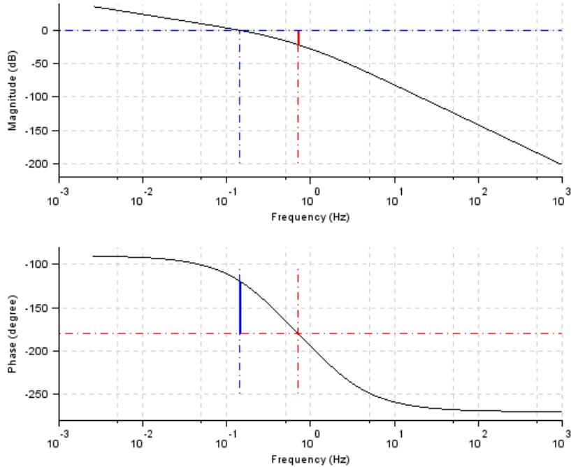
Figure 13.3: To obtain Bode plot of given system
