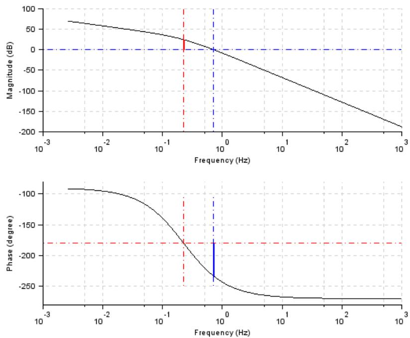
Figure 13.8: To obtain Bode plot of given system
