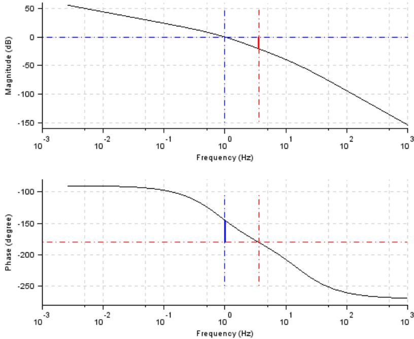
Figure 13.5: To obtain Bode plot of given system
