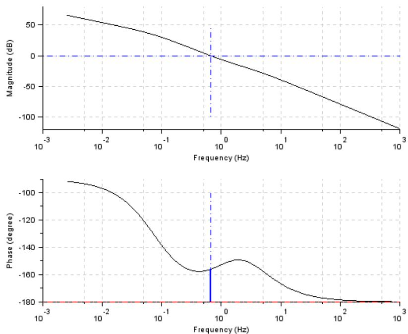
Figure 13.1: To obtain Bode plot of given system
