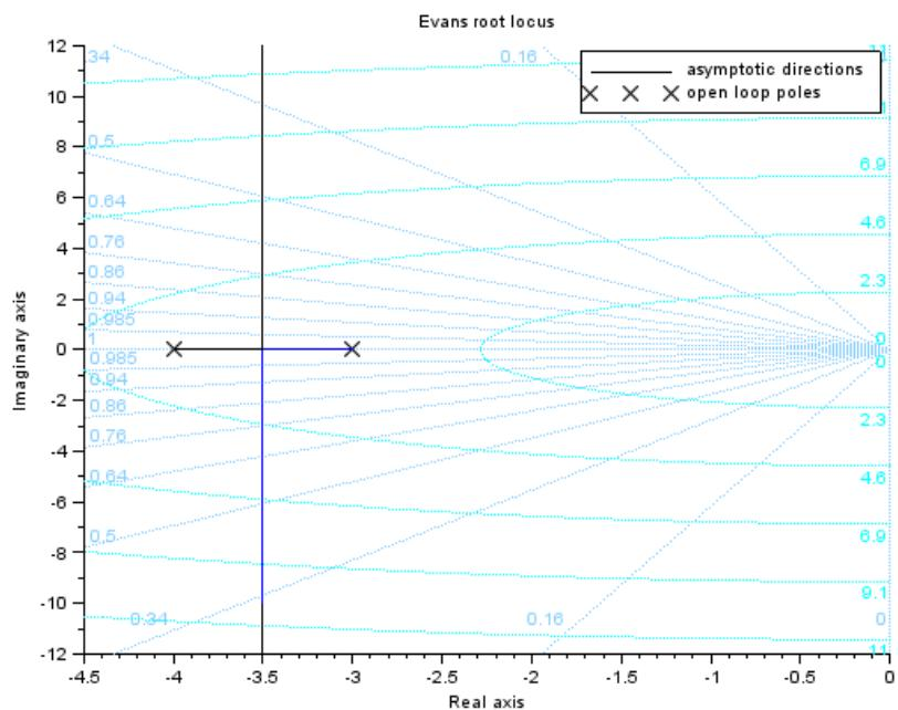
**Scilab code Solution 9.4** To sketch Root locus of given system
