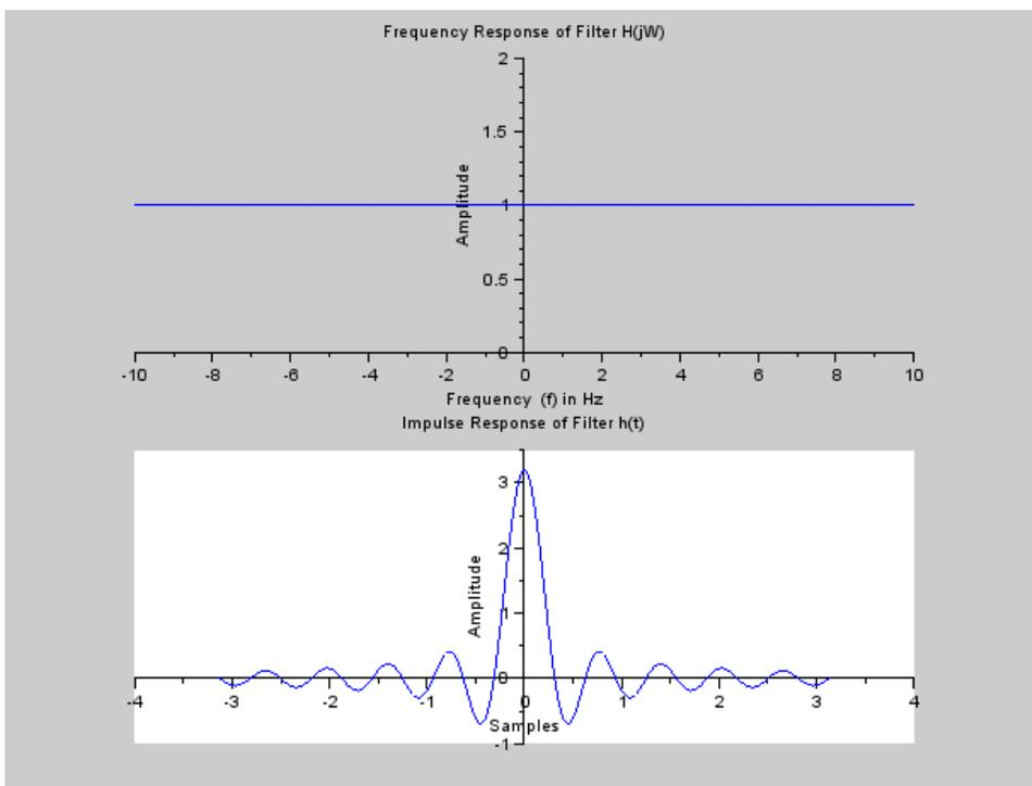
Figure 5.2: Frequency Response of Ideal Low pass Filter
