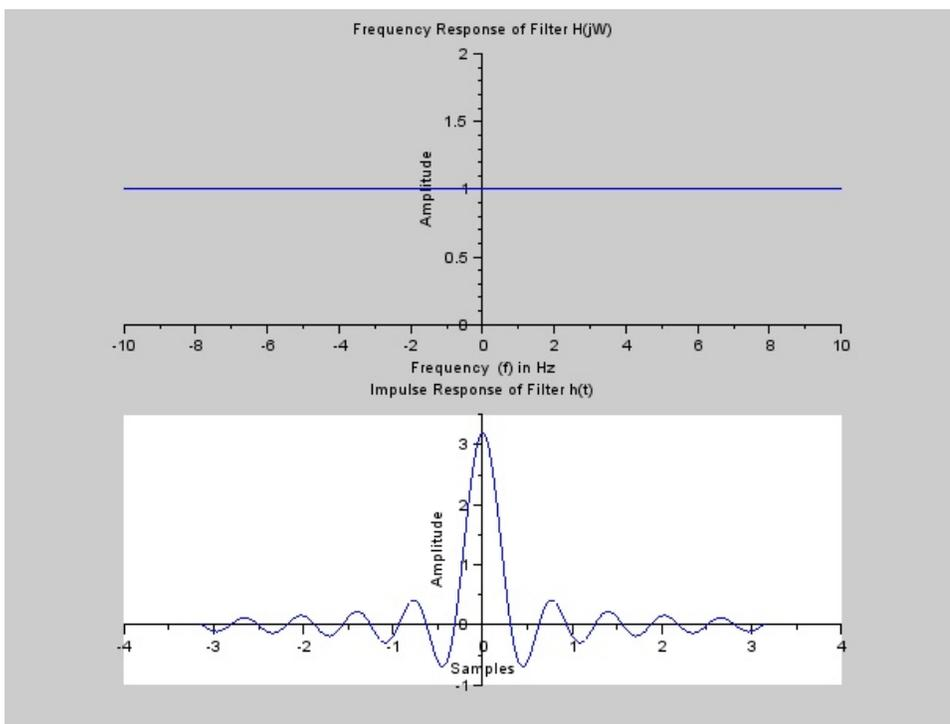
Figure 5.1: Frequency Response of Ideal Low pass Filter
