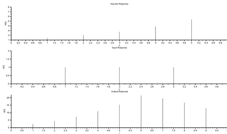
Figure 4.2: convolution sum of finite duration sequences
