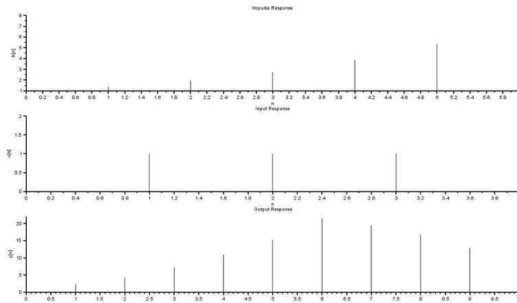
Figure 4.1: convolution sum of finite duration sequences
