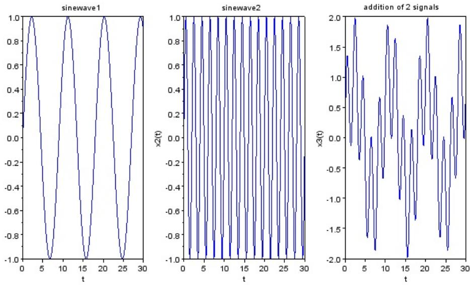
Figure 6.1: Addition of two continuous signals
