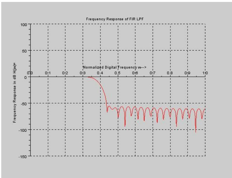
Figure 10.1: To Design an Low Pass FIR Filter
