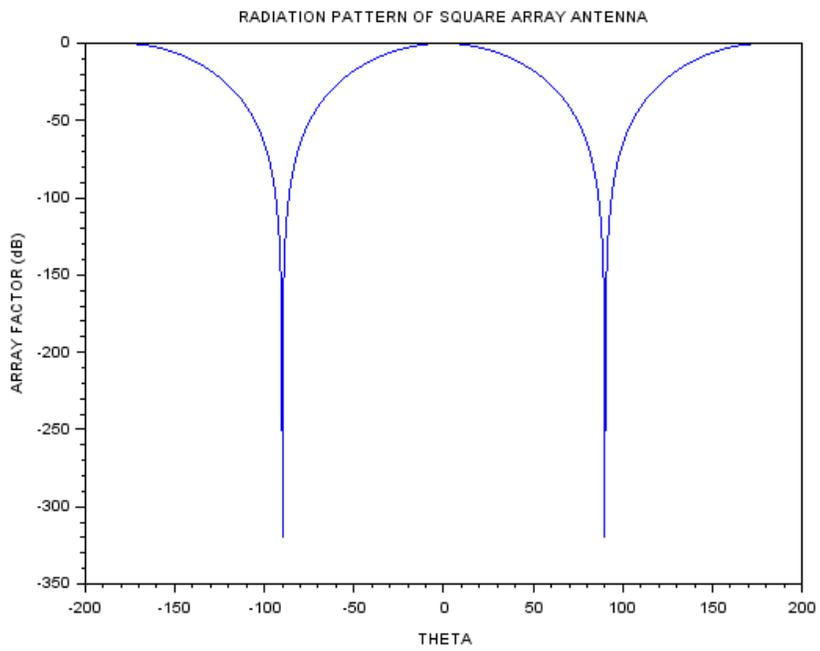
Figure 3.1: Radiation Pattern Measurement of Square Array Antenna
