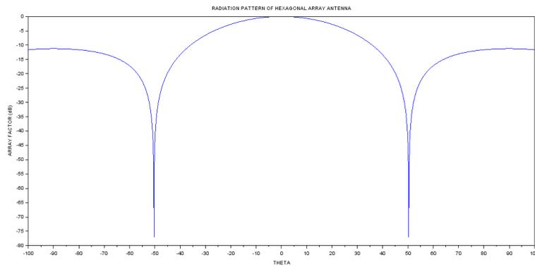
Figure 4.1: Radiation Pattern Measurement of Hexagonal Array Antenna
