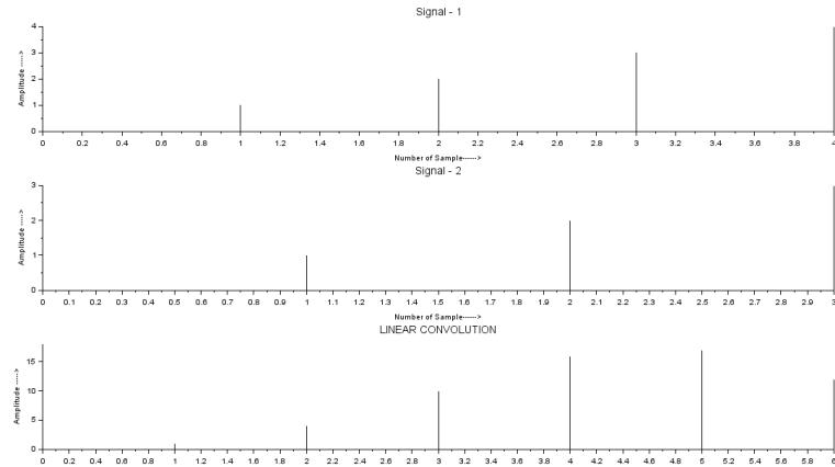
Figure 6.1: Linear Convolution
