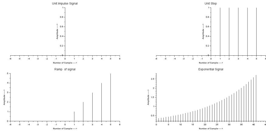
Figure 2.1: Discrete wave with positive exponential
