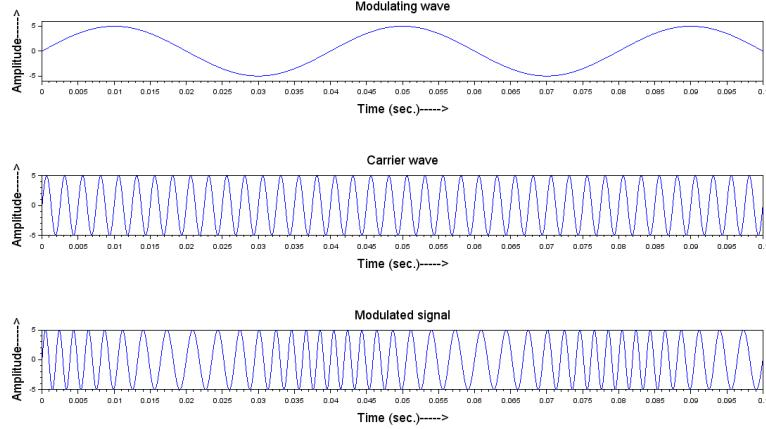
Figure 13.1: Frequency Modulation
