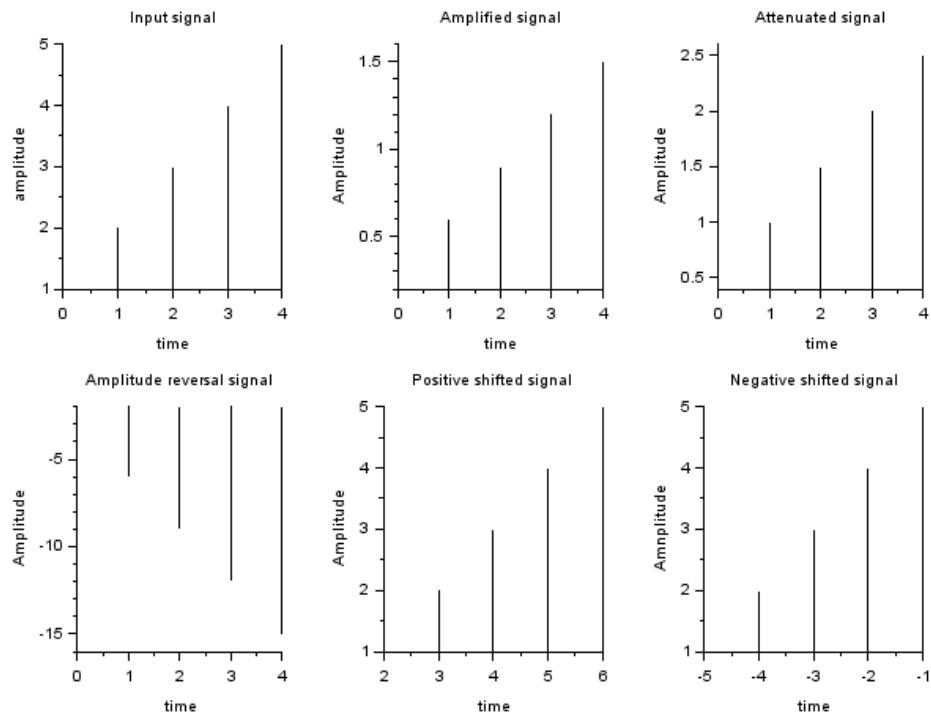
Figure 3.1: TO PERFORM BASIC OPERATIONS ON DT SIGNALS
