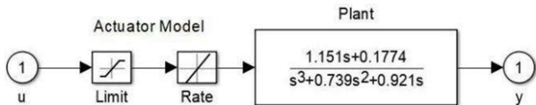
**Figure-** The Block diagram of the Plant – Actuator system
