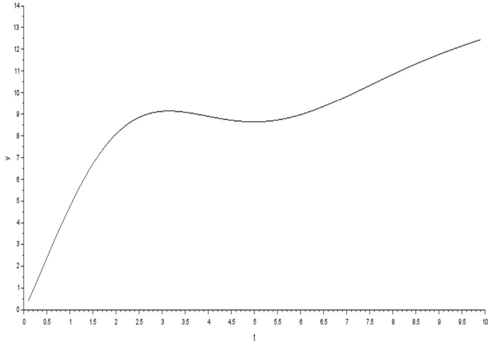
**Figure-** Retaliation of Aircraft pitch control with a gain of  $-0.005$
