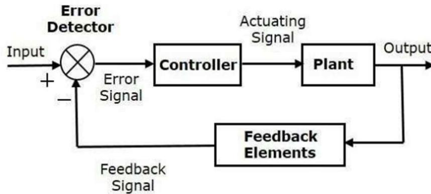
**Figure-** The Block diagram of a closed loop system
