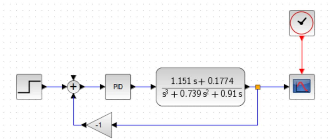
**Figure-** Xcos PID Controller system
