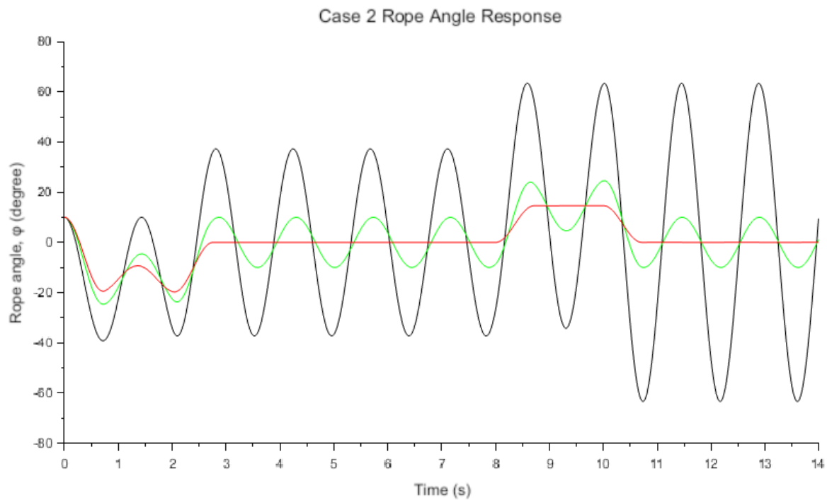
Figure 10. Case 2 rope angle response for unshaped, standard ZV-shaped, and modified ZV-shaped inputs
