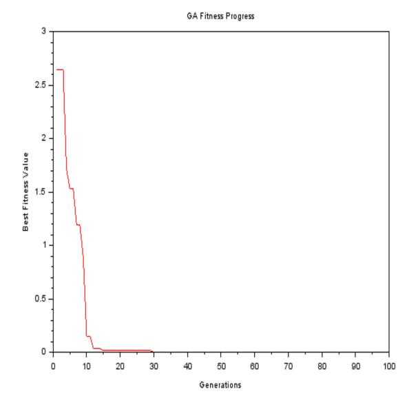
This graph shows the convergence behavior of the Genetic Algorithm over multiple generations. The y-axis represents the best fitness (objective function value) found in each generation, while the x-axis denotes the generation count. A downward trend indicates that the algorithm is successfully finding better solutions over time.
