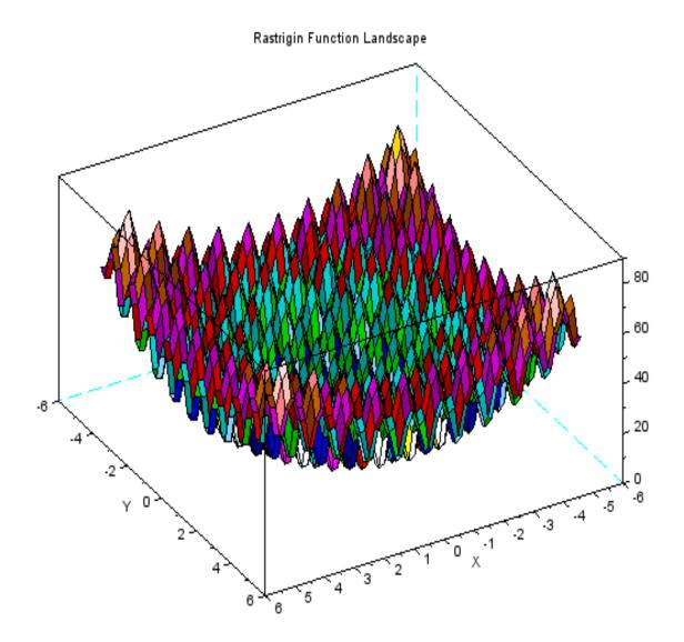
This 3D surface plot visualizes the Rastrigin function, known for its non-convex, multimodal nature. The surface reveals numerous local minima, making it a challenging test function for optimization algorithms. The global minimum is located at the center of the plot, where all variables are zero.
