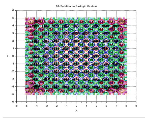
This 2D contour plot provides a top-down view of the Rastrigin function. The contours represent levels of equal objective values. The red marker indicates the best solution found by the Genetic Algorithm, showing how it navigated the complex search space toward the global minimum.
