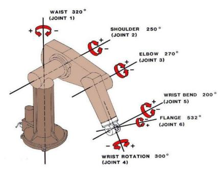
The PUMA (Programmable Universal Machine for Assembly) 560 is an industrial robotic system, also notable for being the first surgical robotic arm (1985). The PUMA 560 model is available in the Robotics Toolbox for Scilab, which is inspired by the ninth release of the Robotics Toolbox for MATLAB by Peter Corke.
