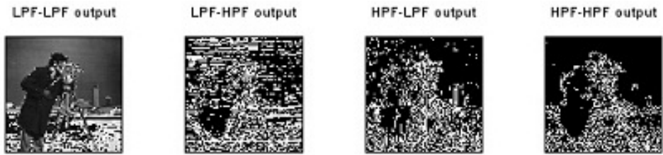
Figure 4.1: DWT and IDWT of 2D Image
