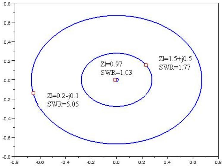
Figure 4.1: To plot SWR circle for an impedance
