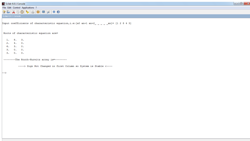
Figure 6.1: Routh Stability Criterion
