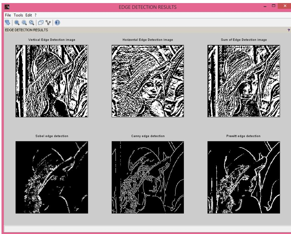
Figure 5.3: To study and perform various segmentation techniques
